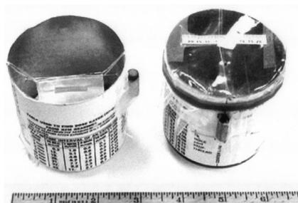
**Figure 2.** Completed KFM units. (left) Construction of the first unit, completed by first year engineering undergraduate, took over 5 h to complete. (right) The second unit, completed by a fourth year engineering undergraduate, required nearly 3 h using the experience and knowledge of the first.
